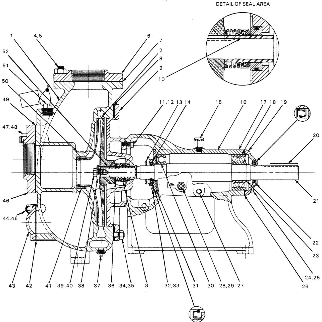
Figure 1. Pump Model 03A52-B
