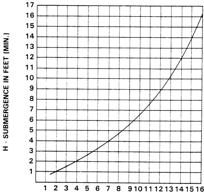
$$\text{VELOCITY IN FEET PER SEC.} = \frac{\text{QUAN. [G.P.M.] x .321}}{\text{AREA}} \text{ OR } \frac{\text{G.P.M. x .4085}}{D^2}$$
