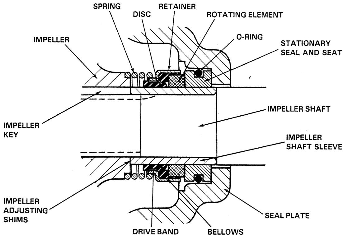
Figure 2. 25284-951 Seal Assembly
