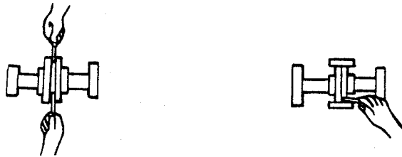
Figure 2B. Aligning Non-Spider Type Couplings
