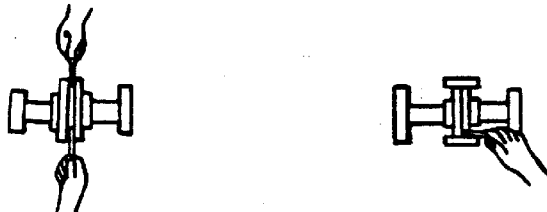
Figure 3B. Aligning Non-Spider Type Couplings
