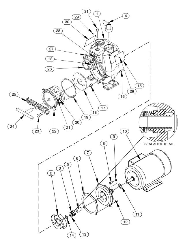
Figure 1. Pump Models 11 1/2A3-KW1.5 3P
