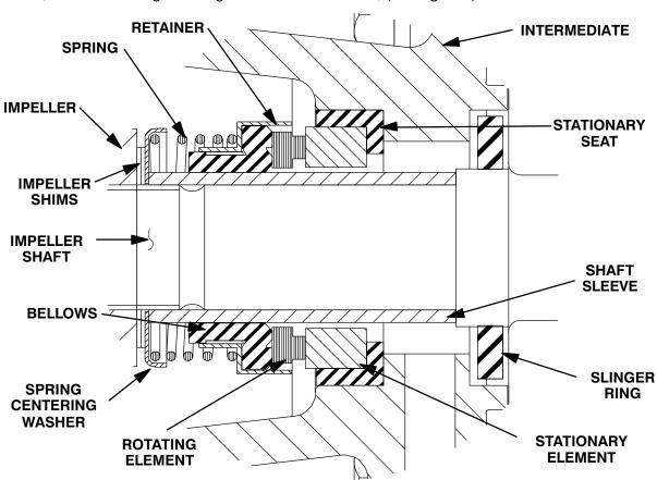
Figure 2. Seal Assembly
