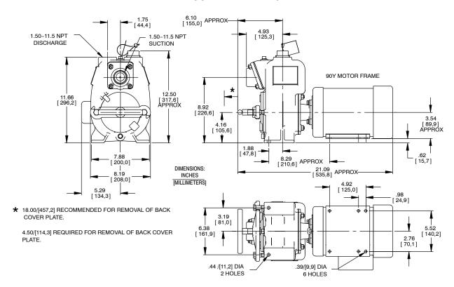
Figure 1. Pump Models 11 1/2A3-KW1.5 3P
