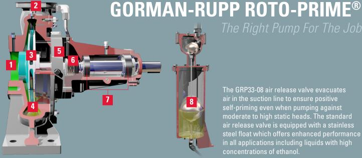
The GRP33-08 air release valve evacuates air in the suction line to ensure positive self-priming even when pumping against moderate to high static heads. The standard air release valve is equipped with a stainless steel float which offers enhanced performance in all applications including liquids with high concentrations of ethanol.
