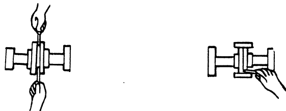
Figure 5A. Aligning Non-Spider Type Couplings
