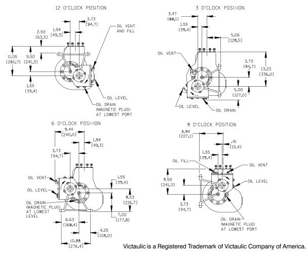
Figure 1. Pump Model 06D17-GAR
