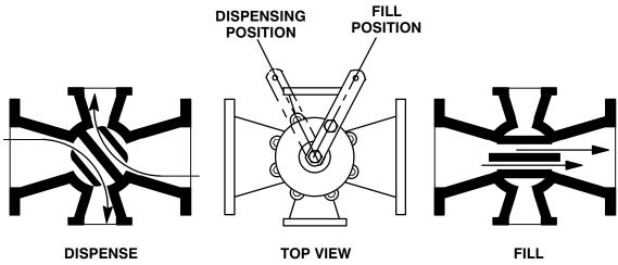
Figure 5. FDF Valve Theory of Operation
