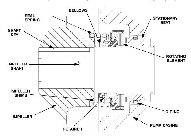
Figure 2. 25271-192 Seal Assembly
